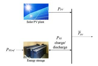
Fig. 2. Operation of ES for PV RR control application.
