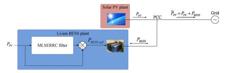
Fig. 6. Implementation of MLSERRC filter for smoothing PV output power [59].
