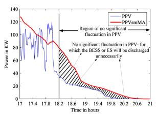
Fig. 11. PV output power smoothing using 51 point MA method for specific hours.
