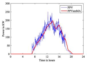
Fig. 10. PV output power smoothing using 51 point MA method.
