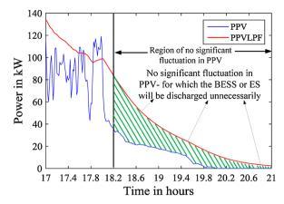
Fig. 15. PV output power smoothing using LPF method for specific hours.
