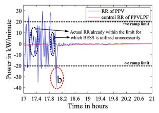
Fig. 17. RR control ability of LPF method for specific hours.
