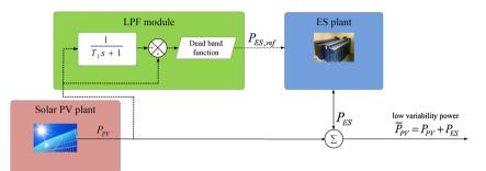
Fig. 5. Typical implementation of LPF filter for smoothing PV plant output power.
