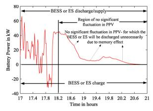
Fig. 12. BESS utilization for 51 point MA method for specific hours.
