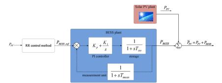
Fig. 8. Implementation of RR control strategy through dynamic model of PV-BESS system [71].
