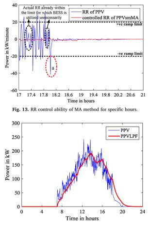
Fig. 14. PV output power smoothing using LPF.
