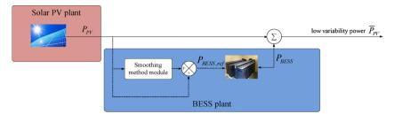
Fig. 4. Generalized implementation of BESS for smoothing PV plant using MA.
