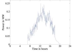
Fig. 1. Typical output power from PV observed using 1-min radiation data.
