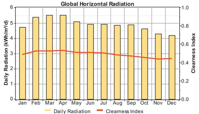
Fig. 5. Monthly average solar radiation (kWh/m<sup>2</sup>/d) over Malaysia.
