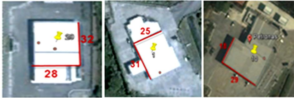
Fig. 3. Sample of estimated net roof area of PETRONAS stations by using Google image.
