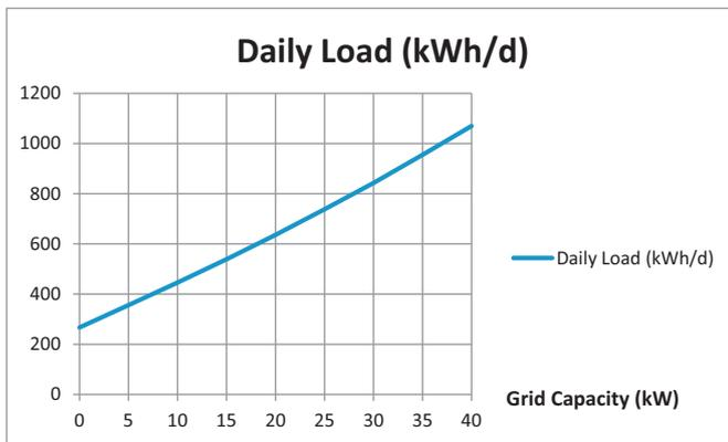
Fig. 7. Linear relation between grid capacity and daily charging load.
