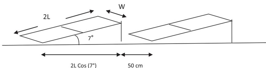
Fig. 6. Flat roof area required for installing a string of two PV panels tilted at 7° and a part 50 cm from next sup array.
