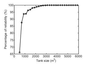
Fig. 8. Percentage of reliability against tank sizes for the large commercial building.
