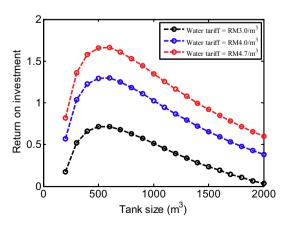
Fig. 6. Effects of tank size on the ROI for of the proposed RWHS for the small commercial building.
