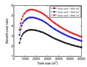
Fig. 11. Effects of tank sizes on the BCR of the proposed RWHS for the large commercial building.
