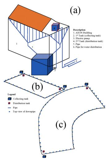
**Fig. 1.** (a) A side view of the proposed RWHS design, (b) plan view of the tank location and downpipe for small building, and (c) plan view of the tank location and downpipe for large building.
