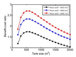
Fig. 7. Effects of tank sizes on the BCR of the proposed RWHS for the small commercial building.
