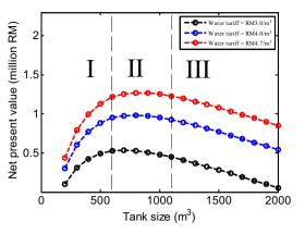
Fig. 5. Effects of tank size on the NPV of the proposed RWHS for the small commercial building.
