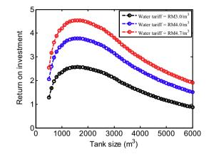
Fig. 10. Effects of tank size on the ROI for of the proposed RWHS for the large commercial building.
