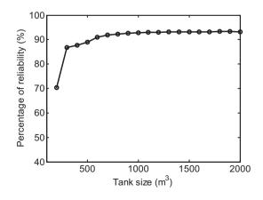
Fig. 4. Percentage of reliability against tank sizes for small commercial building.
