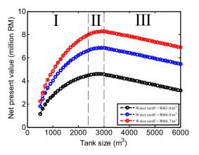
Fig. 9. Effects of tank size on the NPV of the proposed RWHS for the large commercial building.
