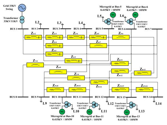
Fig. 1. VPP system includes the IEEE 14-bus test system and five MGs.
