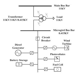
Fig. 3. Single-line diagram of the developed MG system.
