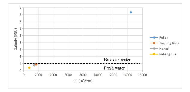
Figure 4. Salinity vs EC in groundwater samples for all tube well location
