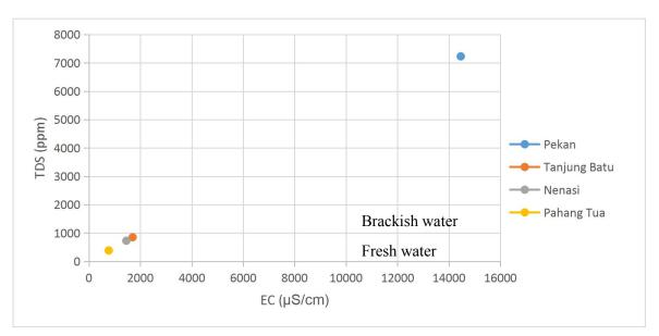
Figure 3. TDS vs EC in groundwater samples for all tube well location
