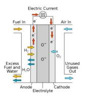
Figure 3. SOFC Basic Operation in automotive application [20].
