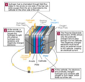
Figure 2. PEMFC Basic Operation [7].
