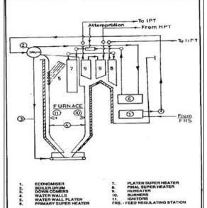
Figure 1: Cross Section of Boiler
