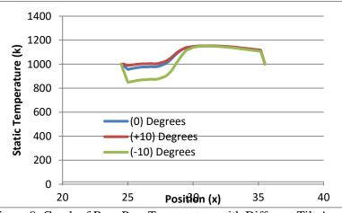
Figure 8: Graph of Rear Pass Temperature with Different Tilt Angle
