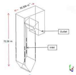
Figure 2: Layout of boiler model
