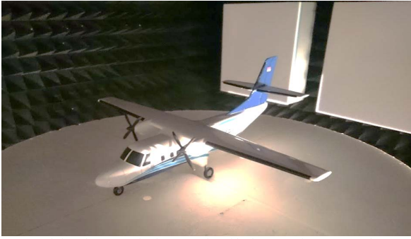
Fig. 9. Model turboprop airplane made of balsa wood as a complex target.
