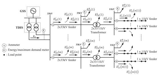
Fig. 1. Representation of energy flow in radial MV distribution network.
