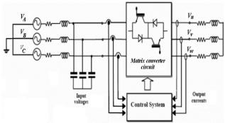
Fig. 2. Practical scheme of matrix converter.
