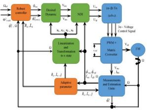
Fig. 3. The dynamic invers controller for induction motor.
