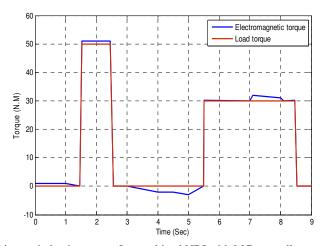
Fig. 8. Torque tracking on induction motor for combined NDI with MC controller.
