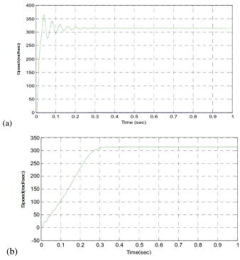
Fig. 6. Induction motor speed: (a) matrix converter without using NDI, (b) with NDI.
