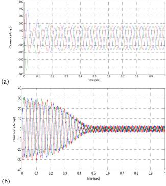
Fig. 4. (a) output current of matrix converter without using NDI, (b) output current with NDI.
