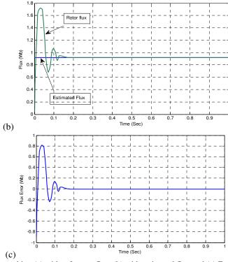
Fig. 10. Rotor flux tracking (a) with reference flux, (b) with estimated flux and (c) Error in tracking.
