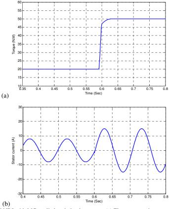
Fig. 9. Combined NDI with MC applied on induction motor: (a) Electromagnetic torque, (b) Stator current.
