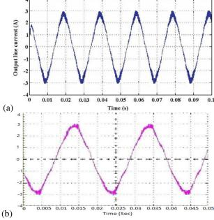
Fig. 11. Output line current: (a) simulation, (b) experimental.
