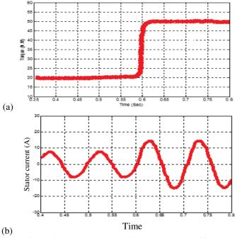
Fig. 12. Experimental result: (a) electromagnet torque, (b) stator current tracking.
