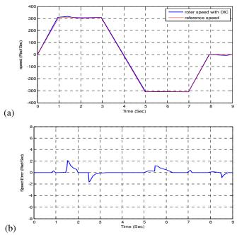
Fig. 7. Combined NDI with MC applied on induction motor: (a) speed tracking, (b) speed error.
