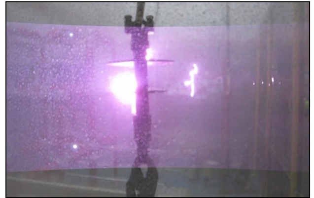
Fig 7: Flashover path of contaminated insulator during polluted air test
