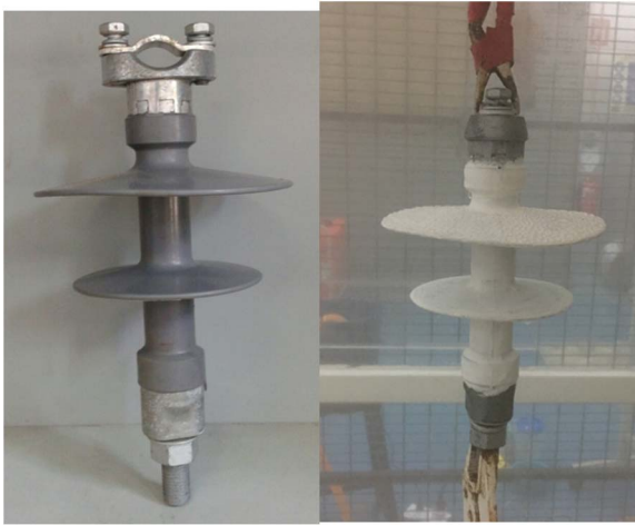
Figure 1. (a) 10 kV Polymer Insulator (b) 10 kV Polymer Insulator with Coating
