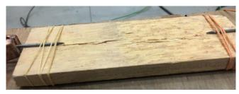
Figure 3: Bentonite contaminated sample with parallel fiber orientation before and after 25 voltage impulses (12 breakdowns)
