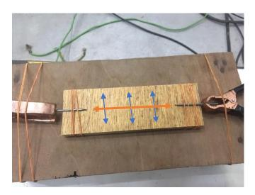
Figure 1: Dry sample with no contamination setup for perpendicular fiber orientation
