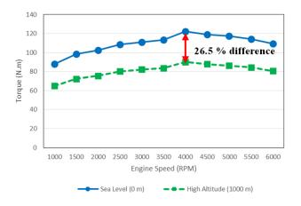
Figure 5. Comparison of engine torque at sea level (0 m) and high altitude (1000 m)
