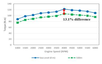
Figure 3. Comparison of engine torque at sea level (0 m) and high altitude (500 m)
