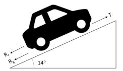
T = Traction force on wheels (in N)  $R_{\rm I} = Rolling \ resistance \ (in N)$ R = Gradient resistance (in N)
