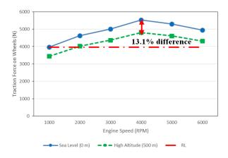
Figure 4.Comparison of traction force on wheels at sea level (0 m) and high altitude (500 m)
