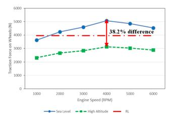
Figure 8. Comparison of traction force on wheels at sea level (0 m) and high altitude (1500 m)
