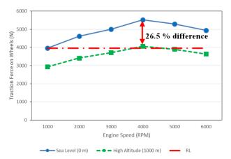
Figure 6. Comparison of traction force on wheels at sea level (0 m) and high altitude (1000 m)
