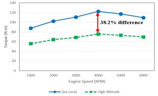
Figure 7. Comparison of engine torque at sea level (0 m) and high altitude (1500 m)
