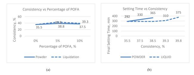
FIGURE 3. (a) Graph of Relationship between Consistency and Percentage of POFA (b) Graph of Relationship between Setting Time and Consistency
