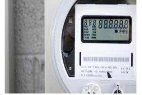
Fig. 5: A sample of AMI used to notify occupants in real time mode and calculate energy cost [31]
