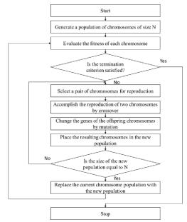
Fig. 2. Flow chart for genetic algorithm approach.
