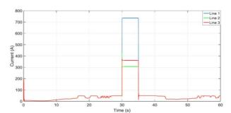
Fig. 6. Current flow through OCR12 during single line to ground fault.
