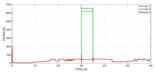
Fig. 7. Current flow through OCR12 during line-to-line fault.
