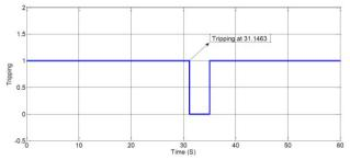
Fig. 15. OCR2 trips during fault incidence
