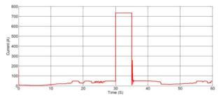
Fig. 8. Current flow through OCR12 during 3-phase fault.
