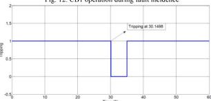
Fig. 13. OCR12 trips during fault incidence
