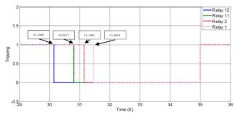
Fig. 17. Coordination of OCRs for fault occurrence
