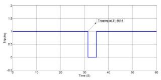
Fig. 3. OCR1 trips during fault incidence
