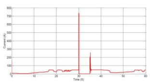
Fig. 9. CB12 operation during fault incidence
