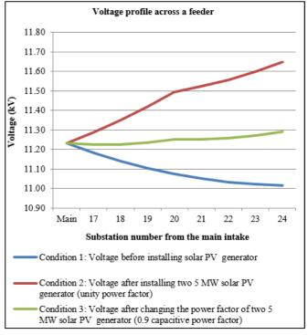
Fig. 4. Voltage Profile across the Feeders in Case 3
