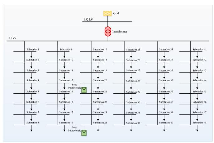
Fig. 1. A distribution network designed using DIgSILENT software
