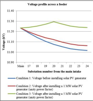
Fig. 2. Voltage Profile across the Feeders in Case 1
