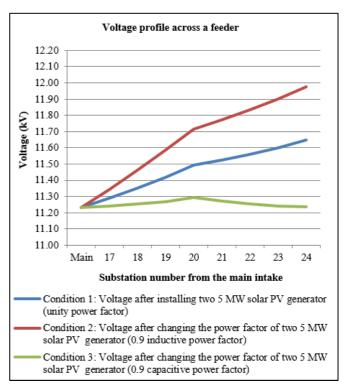
Fig. 5. Voltage Profile across the Feeders in Case 4
