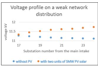
Fig. 6. Voltage Profile for Weak Network Distribution
