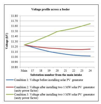
Fig. 3. Voltage Profile across the Feeders in Case 2
