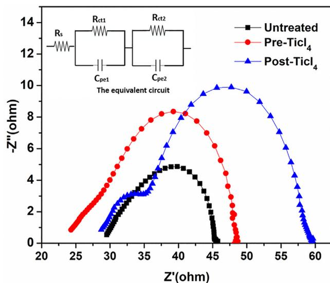
Fig. 5. Nyquist plot of treated, pre-TiCl<sub>4</sub>, and post TiCl<sub>4</sub> treatment with the equivalent circuit (inlet) represent the impedance of the cell; sheet resistance R<sub>s</sub>, electrochemical capacitance C<sub>pe</sub> and charge transfer resistance R<sub>ct</sub>.
