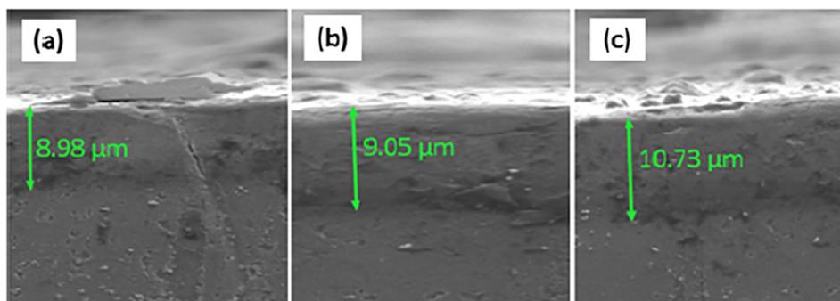
Fig. 2. Cross-sectional SEM images of thickness on (a) untreated (c) pre- $\text{TiCl}_4$  treatment and (e) post- $\text{TiCl}_4$  treatment on photoelectrodes.
