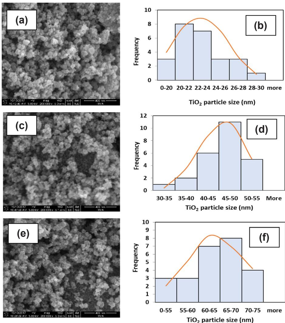
Fig. 3. FESEM morphology of particle necking and distribution of TiO<sub>2</sub> nanoparticle with the Gaussian fitting curve (orange line) of (a)(b): Untreated electrode, (c) (d): pre-TiCl<sub>4</sub> treatment, and (e)(f): Post-TiCl<sub>4</sub> treatment photoelectrode, respectively. (For interpretation of the references to colour in this figure legend, the reader is referred to the web version of this article.)
