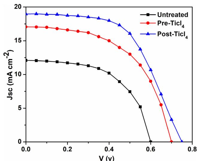
Fig. 8. J–V curve for DSSC of untreated, Pre-TiCl<sub>4</sub>, and Post-TiCl<sub>4</sub>.
