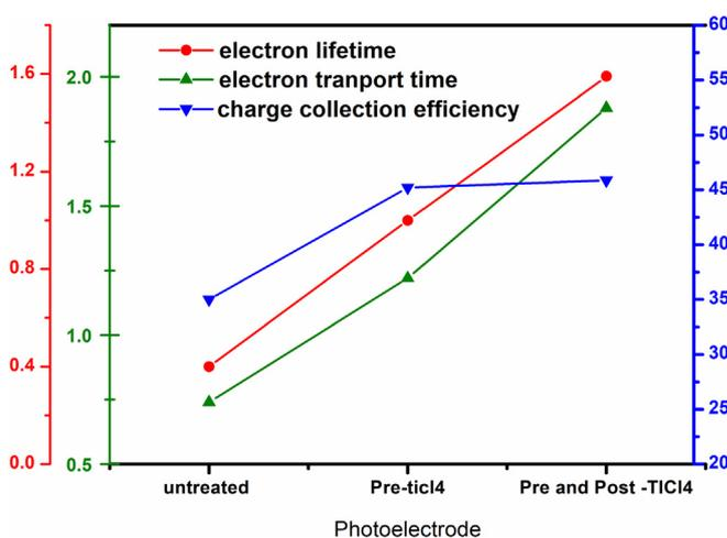
Fig. 7. Comparison of electron lifetime  $\tau_n$ , electron transport time  $\tau_s$ , and charge collection efficiency  $\eta_c$  for untreated, pre-TiCl<sub>4</sub>, and post-TiCl<sub>4</sub> photoelectrode of DSSC.
