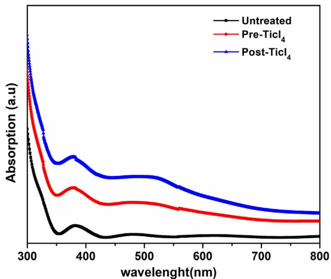
Fig. 4. Absorption spectra of untreated, pre-TiCl<sub>4</sub>, and post-TiCl<sub>4</sub> treatment on TiO<sub>2</sub> film after N-719 dye sensitising.
