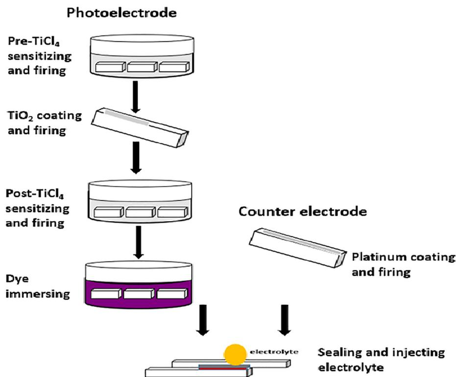
Fig. 1.  $\text{TiCl}_4$  treatment and DSSC fabrication process.
