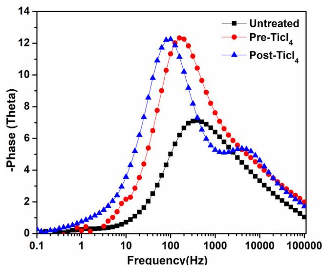
Fig. 6. Bode plot of treated, pre-TiCl<sub>4</sub> and post-TiCl<sub>4</sub>.
