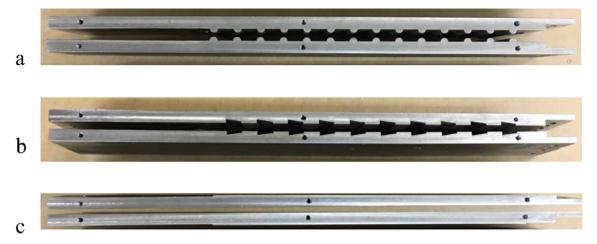
Fig. 7. Front view of different shapes of test modules (a) semicircle module, (b) trapezoidal module, and (c) straight module.
