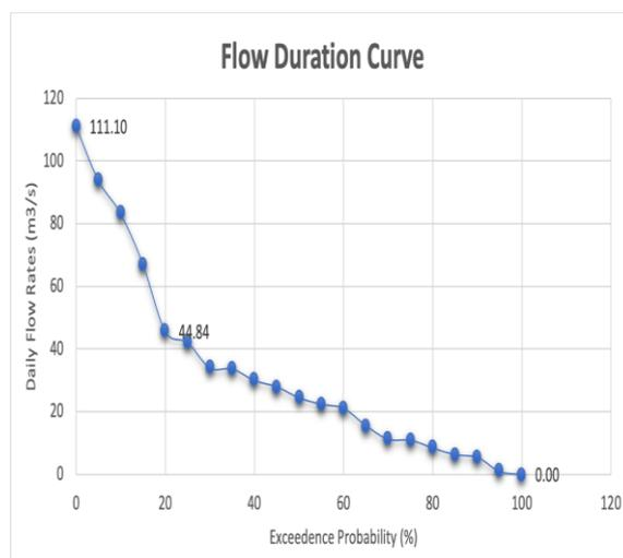
Fig. 6 Flow duration curve for Pedu Dam for 2017
