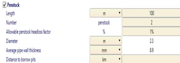
**Fig. 7** Estimated value suggested by the software for penstock dimensions
