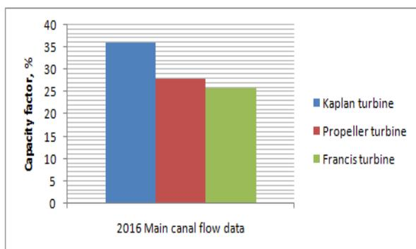
**Fig. 11 Plant Capacity Factors using different turbine types**
