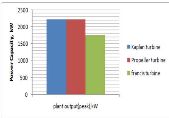
**Fig. 9 Plant power capacities using different turbine types**
