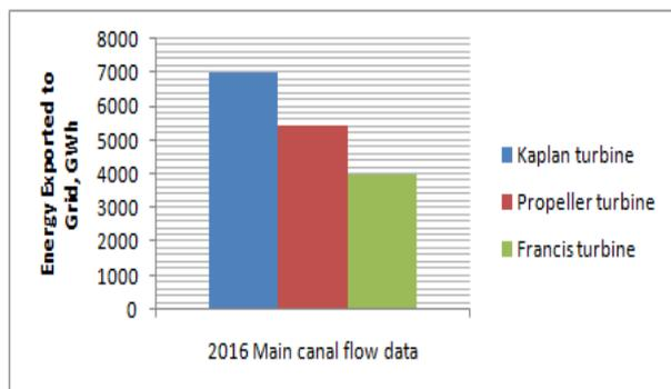
**Fig. 10 Energy output using different turbine types**
