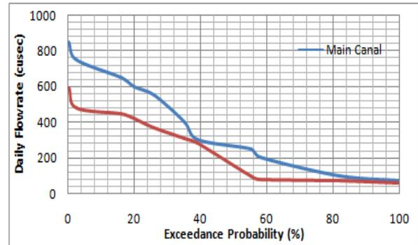
Fig. 8 Comparison of flow duration curve between the Main Canal and Selinsing Canal for 2016 daily flow rate data
