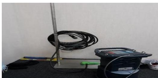
**Fig. 1 HACH FL900 portable ultrasonic water flow sensor with data logger**
