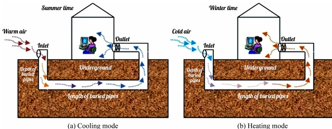
Fig. 12. Conceptual view of (a) cooling and (b) heating modes of EATHE. Reproduced from [Singh et al. \(2018\)](#).
