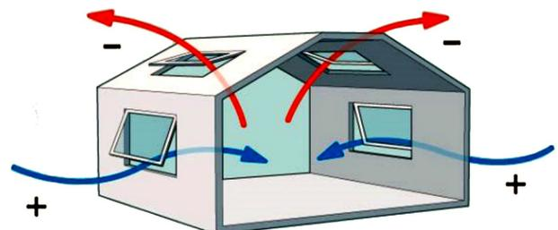
Fig. 7. Schematic diagram of the stack ventilation approach. Reproduce from <https://www.tealproducts.com/natural-ventilation-control>
