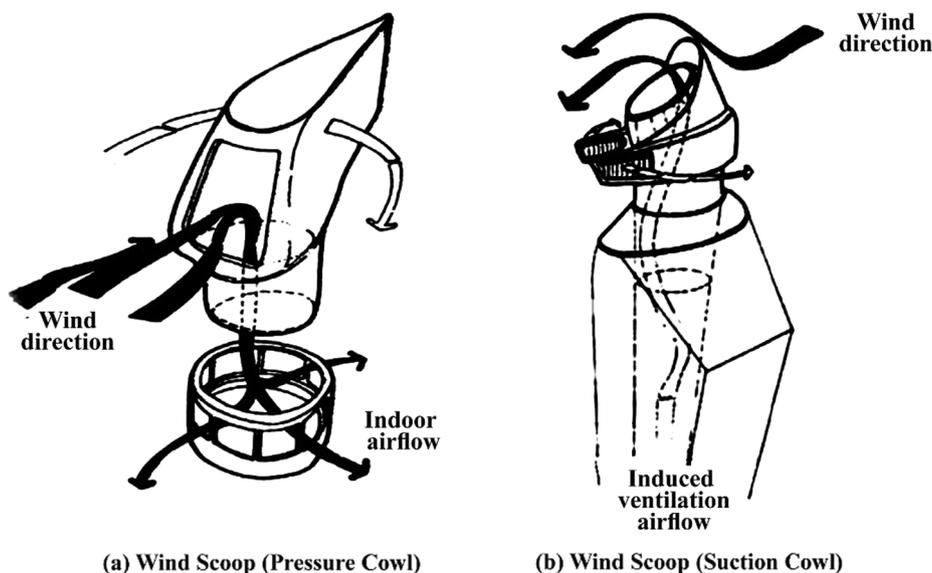
Fig. 10. Schematic examples of pressure cowl and suction cowl retrieved from Khan et al. (2008).
