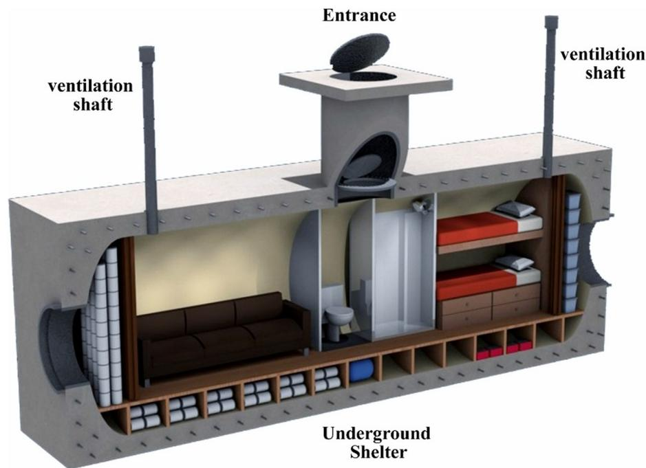
Fig. 8. The use of vertical ventilation shaft for the ventilation system in an underground shelter. Reproduce from <https://bornprepper.com/build-underground-bunker/>
