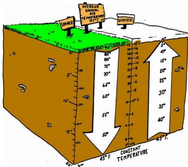
Fig. 4. The soil temperature equals to the average annual air temperature at depth of 20 ft. Reproduced from Hait (1983).
