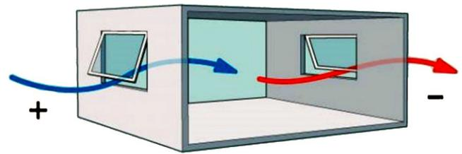
Fig. 6. Schematic diagram of the cross-ventilation approach. Reproduce from <https://www.tealproducts.com/natural-ventilation-control>
