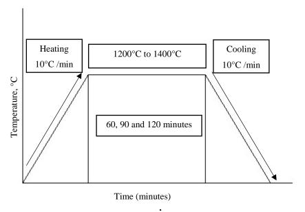
Figure 1: Graph of Sintering profile
