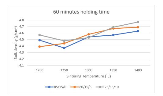
Figure 2: The effect of Bulk density on sintering temperature for 60 minutes holding time
