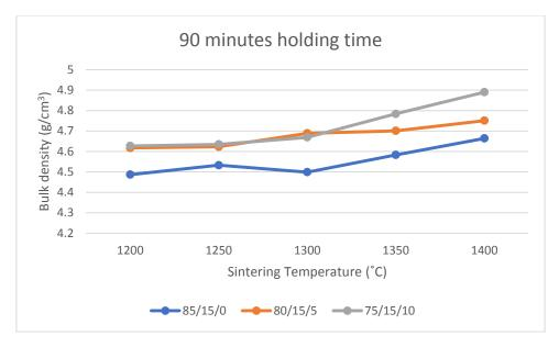
Figure 3: The effect of Bulk density on sintering temperature for 90 minutes holding time
