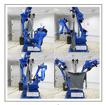
Figure 5. Robot unfolding a shirt.<sup>69</sup>
