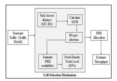
Figure 3. Block diagram of cell selection process
