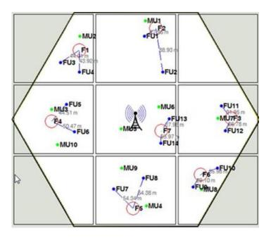
Figure 2. Simulation model for femto-macro heterogeneous network environment
