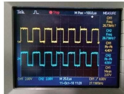
Figure 5. Output signal from DSP TMS320F28335
