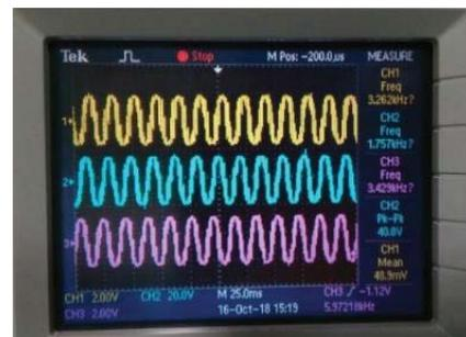
Figure 6. Output signal after low pass filter
