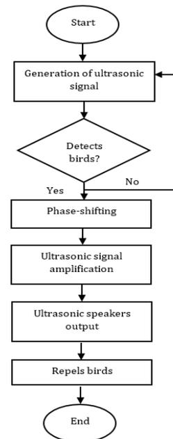
Figure 2. Flowchart of Phased-Array Ultrasonic Bird Deterrent System
