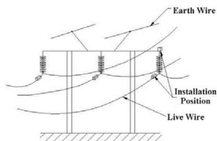
Figure 1. Bird deterrent system at transmission line [1]
