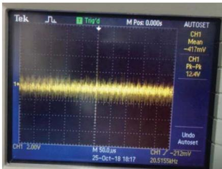
Figure 8. Ultrasonic signal waveform at receiver without beamforming.
