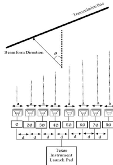
Figure 4. Phase Array transducer arrangement
