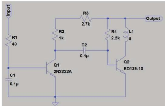
Figure 3. Design of an amplifier circuit
