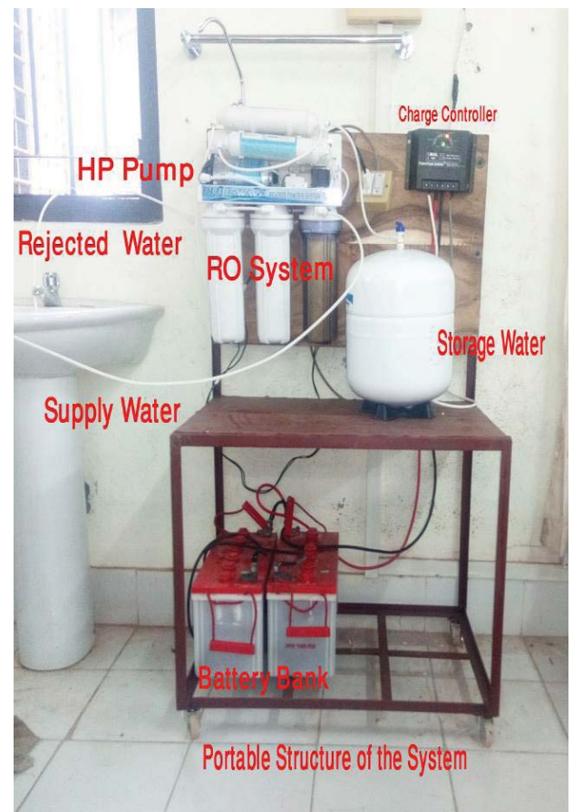
Fig 2 Experimental setup of the prototype
