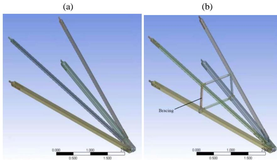
**Figure 1.** The 3-D model of: (a) the cross arm and; (b) cross arm with bracing
