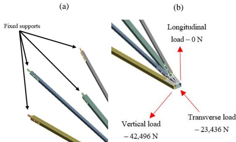
**Figure 2.** Boundary conditions for: (a) fixed supports; (b) load applied
