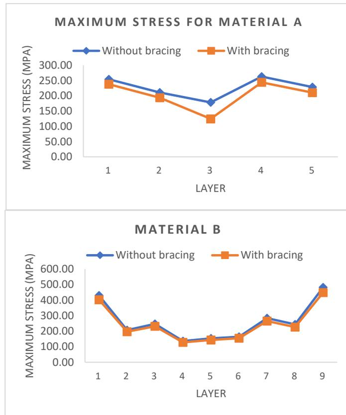
**Figure 3.** Maximum stress recorded for material A and B at each layer.
