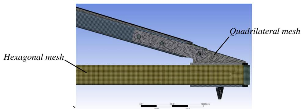
**Figure 1.** The adaptive hybrid mesh that being implemented on the cross arms numerical model.
