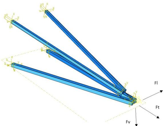
**Figure 2.** FE model of electric power grid substation structure.
