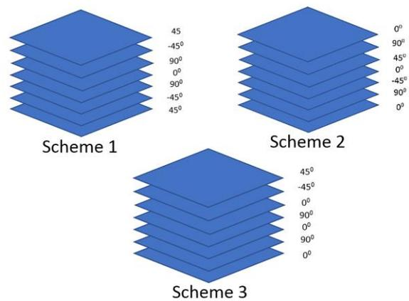
**Figure 3.** Different stacking sequences.
