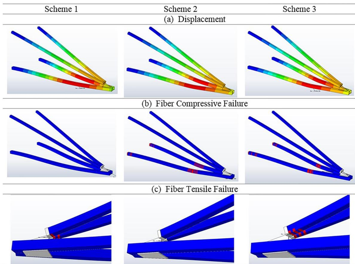
**Figure 4.** Numerical results (a) Displacement contour (b) Fiber compressive failure location (c) Fiber tensile failure location.
