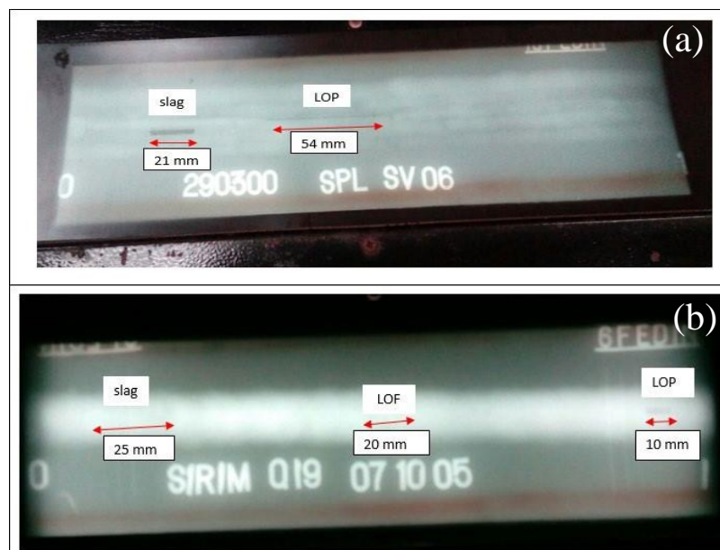
Figure 12. Result of X-ray for (a) Single-V and (b) Double-V
