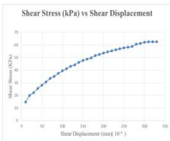
Figure 1. Shear Stress versus Shear Displacement for 2 kg normal load.
