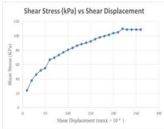
Figure 3. Shear Stress versus Shear Displacement for 6 kg normal load.
