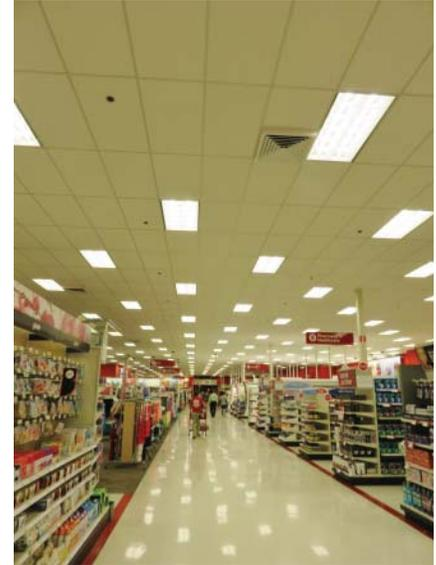
**Figure 5.21** Use of surface reflectance to reduce artificial lighting lamps, fixtures, and energy use. Note the reflective floor and ceiling. This design uses two-lamp T8 fluorescent troffer fixtures, delivering high illuminance at only 0.6 watts per square foot, 60 percent less than the typical lighting power allowance for a sales area.
