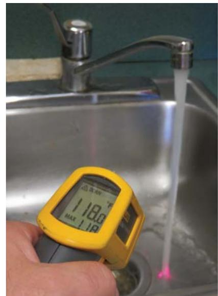
Figure 12.8 Measuring water temperature.
