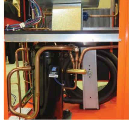
Figure 7.10 Heat pump compressor and reversing valve.
