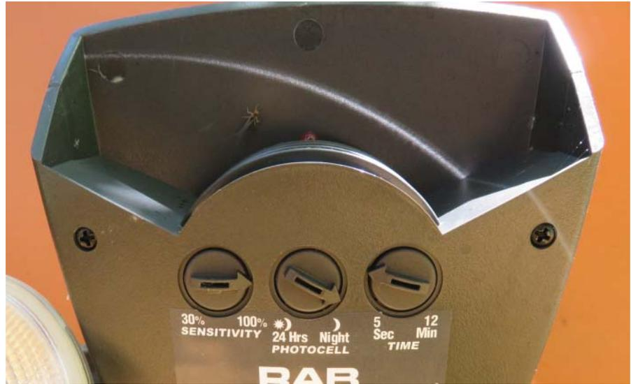
**Figure 5.29** Combined motion and photocell control.
