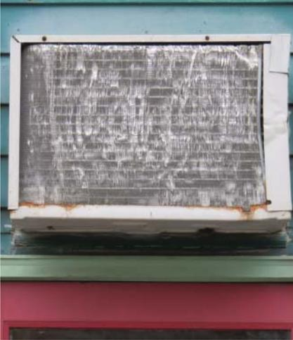
**Figure 3.10** Catastrophic room air conditioner fin damage.
