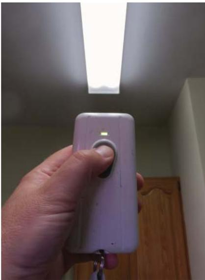
Figure 3.5 Ballast checker.
