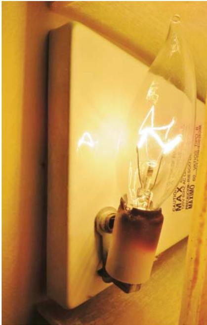
**Figure 5.18** Charred light socket is evidence of an unsafe condition.
