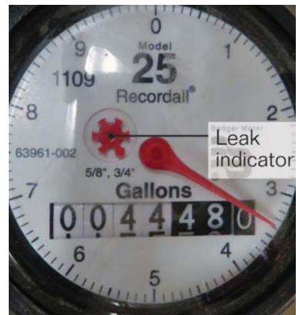
Figure 12.35 Water meter leak indicator.
