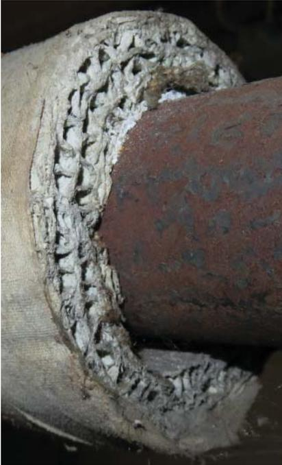
Figure 20.6 Asbestos pipe insulation
