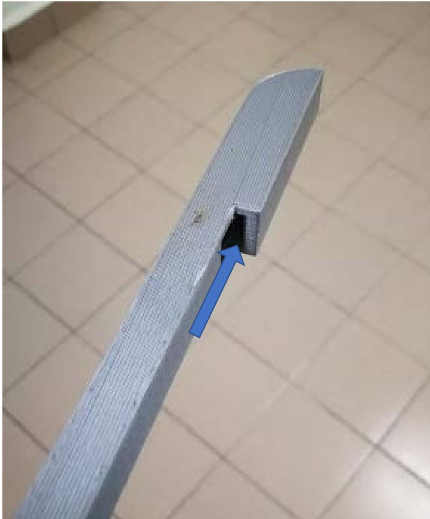
Figure 4.14: Slot design on Prototype 2
