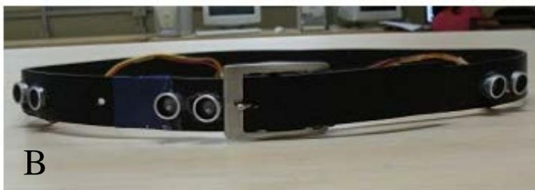
Figure 2.5: (A) Ultrasonic Spectacles (B) Ultrasonic waist belt [36].
