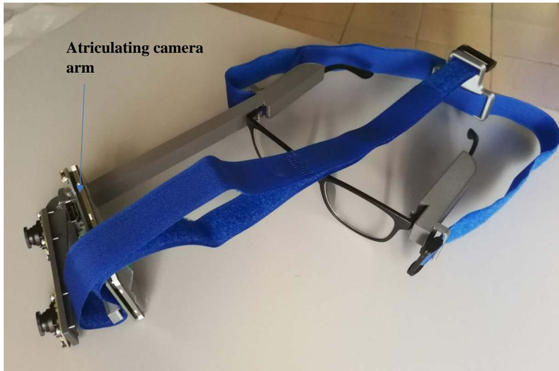
Figure 3.14: Prototype 3 of the visual aid
