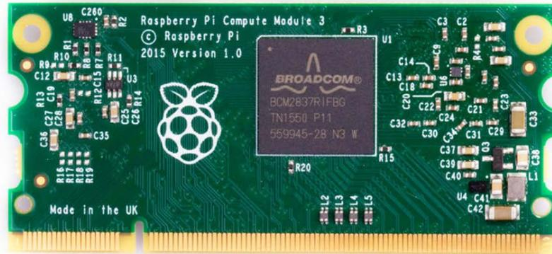
Figure 3.3: Raspberry Pi Compute Module 3 (CM3) [72].
