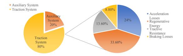
FIGURE 2. Energy consumption distribution in rail transit system
