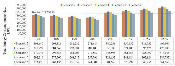
FIGURE 4. Total energy consumption due to headway changes between  $\pm 5\%$  and  $\pm 20\%$
