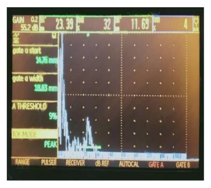
Figure B1.10 Hole Defect Result
