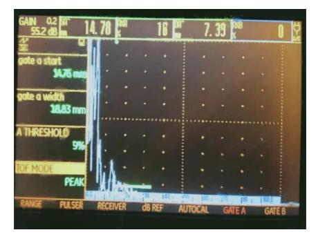
Figure B1.9 Gradient Axial Defect Result
