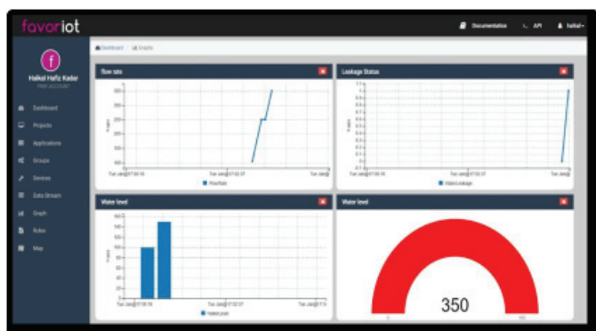
Figure 13: Graphic display of the SMART2L system. The flow rate of the water is shown using a line graph same goes for the leakage status.
