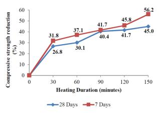
Figure 2. Compressive strength percentage of reduction.
