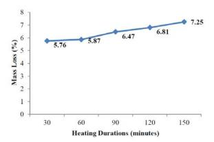
Figure 3. Mass loss of different heating duration.
