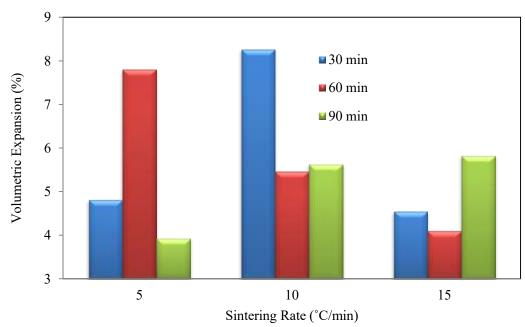
Figure 3. Volumetric expansion (percentage) of samples during sintering.
