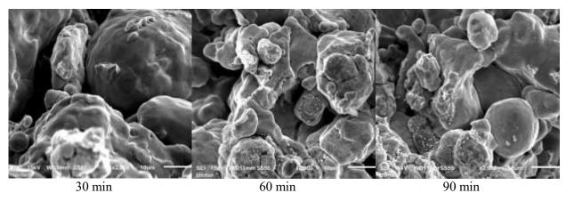
Figure 7. Microstructure of samples sintered at a rate of 10°C/min.
