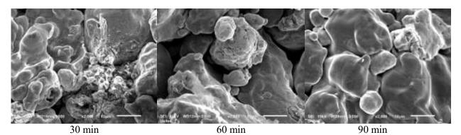
Figure 6. Microstructure of products sintered at a rate of 5°C/min.
