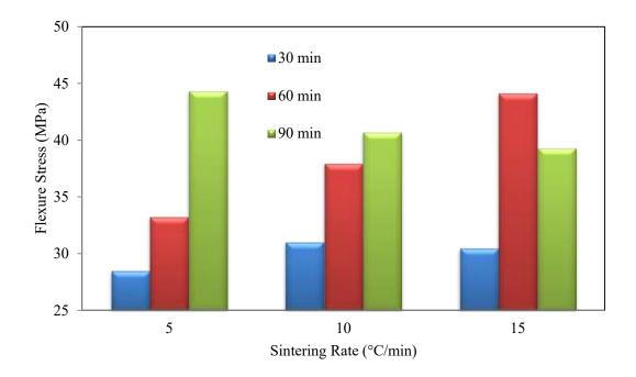
Figure 5. Flexure stress of sintered products.
