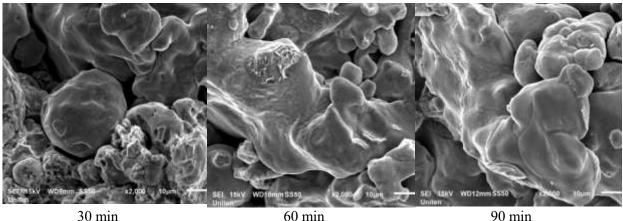
min60 min90Figure 8. Microstructure of samples sintered at a rate of 15°C/min.
