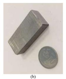
Figure 1. (a). T-15 compaction rig with heating system. (b). FeCuAl green compact.
