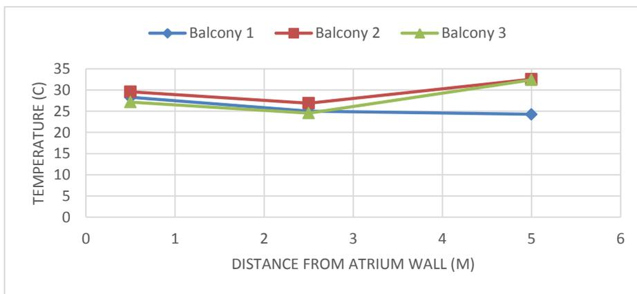
**Figure 3.** Temperature profiles along balcony breadth with solid upstand.
