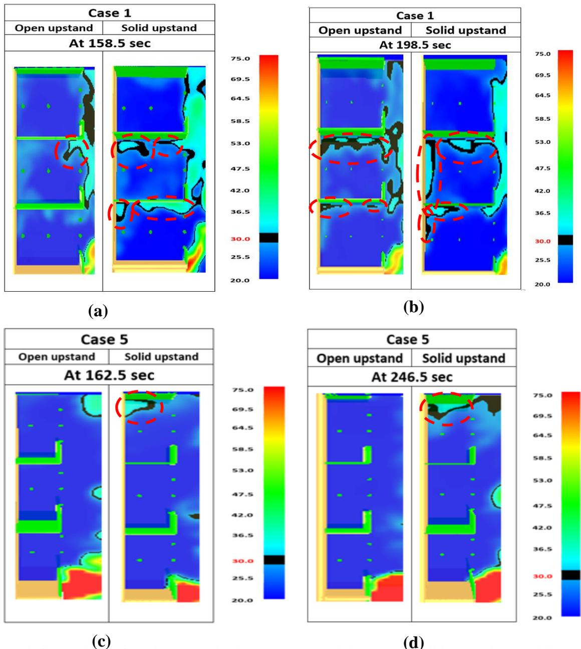
**Figure 6.** Comparison of smoke contamination occurrence with open and solid upstand (a) and (b).
