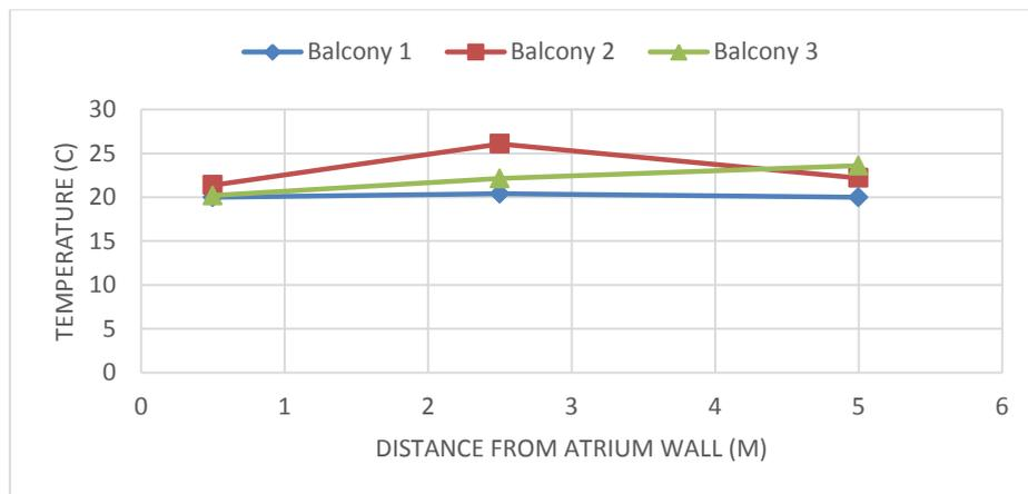
**Figure 4.** Temperature profiles along balcony breadth with open upstand.
