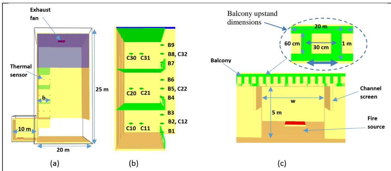
**Figure 1.** Schematic drawing of atrium and fire compartment (a) side view of atrium, (b) Location of temperature sensor, (c) Front view of fire compartment with the balcony upstand.
