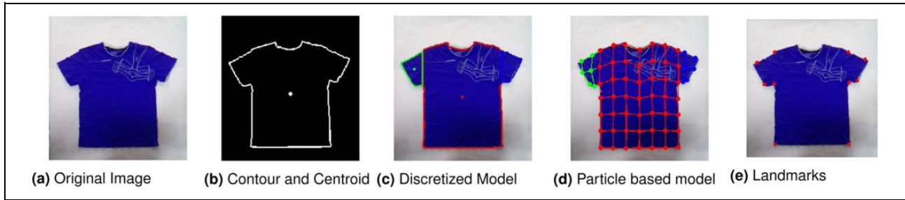
Figure 2. Overview of garment-handling procedure in robotic manipulation process.
