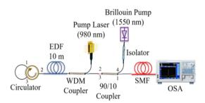
Fig. 1. Experimental setup of multiwavelength BEFL.
