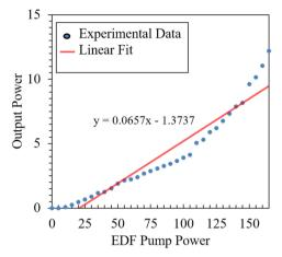
Fig. 2. Evolution of laser output power with EDF pump power.
