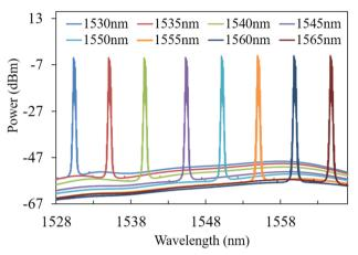
Fig. 4. Tunability of multiwavelength BEFL as a function of BP wavelength.
