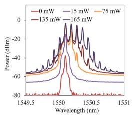
Fig. 3. Spectra of Stokes evolution as EDF pump power increases.
