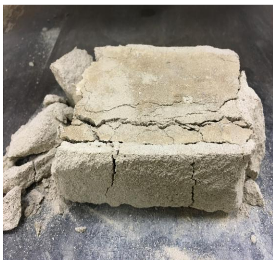
Fig. 14: Brick specimen after compression test
