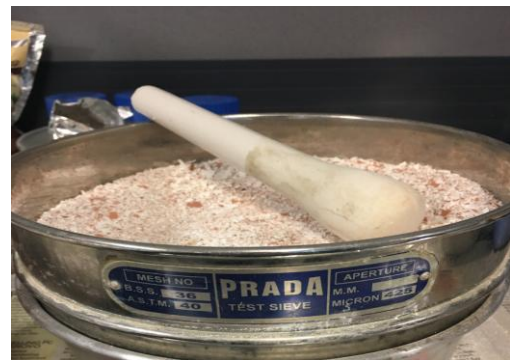
Fig. 4: Grinded eggshell filtered using sieving passing through 425µm pan
