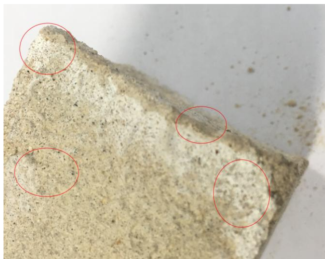
Fig. 11: Evidence of biocementation occur
