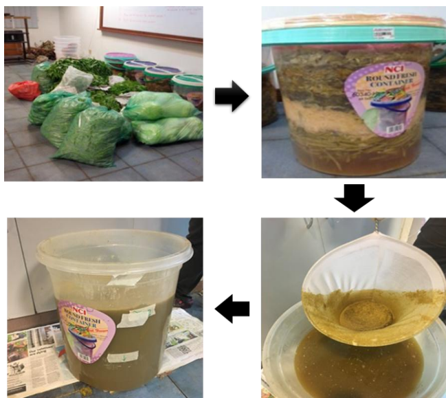
Fig. 1: Fermentation process of vegetables to produce vege-grout liquid
