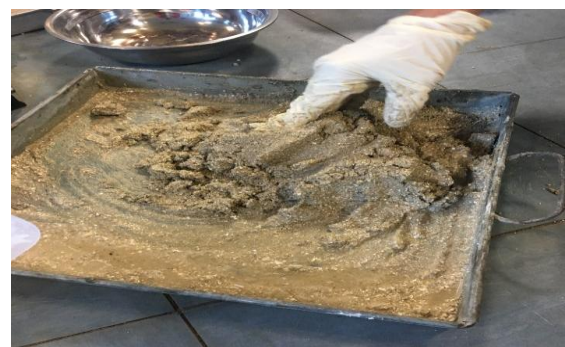
Fig. 5: Hand mixing of soil with vege-grout
