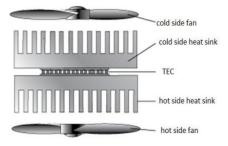
Fig. 2: the configuration of the Peltier thermoelectric cooler. [4]
