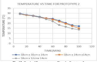
Fig. 15: Graph of Temperature vs. Time for Prototype 2
