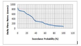
Fig. 6 Daily flow duration curve of Bukit Merah for Main Canal in 2016
