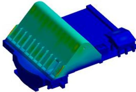
**Figure 7.** ODS of the bottom outlet section.
