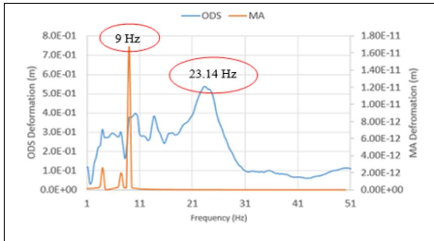
**Figure 10.** Relationship between ODS and MA deformations at the bottom outlet section in frequency domain.
