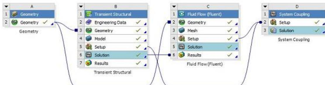
**Figure 6.** Linked setup between systems in two-way FSI.
