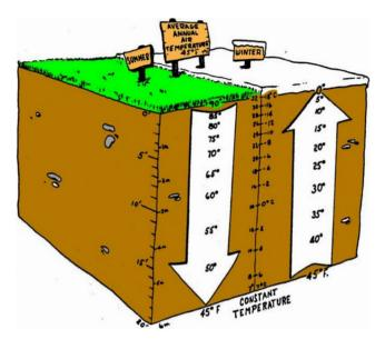
Fig. 4. The soil temperature equals to the average annual air temperature at depth of 20 ft.
