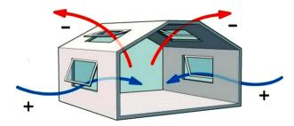
Fig. 7. Schematic diagram of the stack ventilation approach. Reproduce from https://www.tealproducts.com/natural-ventilation-control
