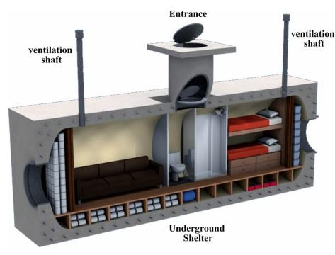
Fig. 8. The use of vertical ventilation shaft for the ventilation system in an underground shelter. Reproduce from https://bornprepper.com/build-underground-bunker/
