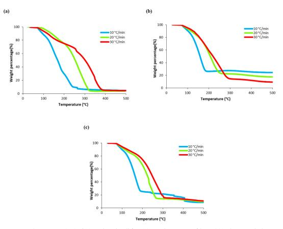
**Figure 1.** Thermogram (TG) of (**a**) *Caulerpa lentillifera*, (**b**) *Gracilaria coronopifolia* and (**c**) *Chaetomorpha linum* at three heating rates (10 °C/min, 20 °C/min and 30 °C/min).
