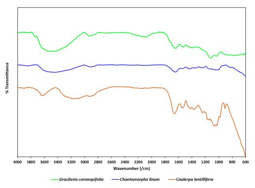
Figure 4. Spectra of algal biomass using FTIR analysis.
