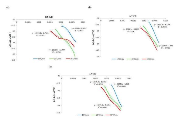
**Figure 3.** Coat-Redfern plot for kinetic parameters determination of (**a**) *Caulerpa lentillifera* (**b**) *Gracilaria coronopifolia* and (**c**) *Chaetomorpha linum*.
